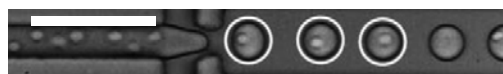
Figure 3: A micrograph depicting the encapsulation of single cells within nanodroplets. The ordering of cells entering the droplet chamber increases the likelihood of a droplet containing a single cell. Scale bar = 150µm. Reproduced from Joensson and Svahn (2012) with permission from Wiley and sons.
