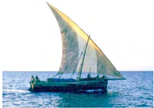
Figure 4. Lateen sail – a semi-conical wing, invented by the Egyptians thousands of years ago.
