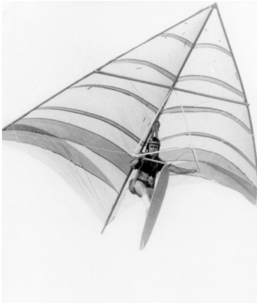
Figure 10. Rod Fuller shows off the wing with the “A” Frame modification, October 1963.
