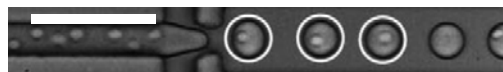
Figure 3: A micrograph depicting the encapsulation of single cells within nanodroplets. The ordering of cells entering the droplet chamber increases the likelihood of a droplet containing a single cell. Scale bar = 150µm. Reproduced from Joensson and Svahn (2012) with permission from Wiley and sons.
