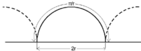
Figure 4: Portion of a section of n semicircular arcs of radius r . The arc length is \pi/r and the diametrical length is 2r , hence the ratio of the arc length to the diametrical length is \pi/2 .
