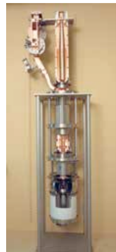
Figure 6: Cutaway view of one of the 240 S-band klystrons delivering up to 65 MW each of peak power at 2856 MHz.
