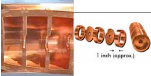
Figure 5: The SLAC linac structure is shown in a cutaway view and comprises roughly 80,000 copper cells.
