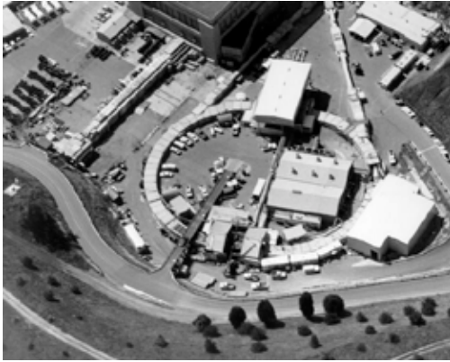
Figure 11: An early photograph of the SPEAR storage ring before it was surrounded by synchrotron radiation hutches.
