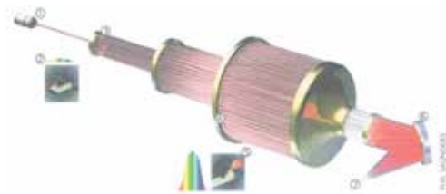
Figure 10. For a new design ICAN (Mourou et al. 2013) of a CPA laser for pulses shorter than 1 ps and with powers of Petawatt to Exawatt and higher, the use of fibres is being designed with an initial partial section for demonstration of highest quality laser pulses on comparably low costs. The beam output of the fibre bundle irradiating a focusing mirror 6 has diffraction limited quality for focusing to highest intensities. It is expected (Mourou 2013) that a cross section of 100 cm 2 ps laser beam may be produced with kJ energy pulse corresponding to a Petawatt power.
