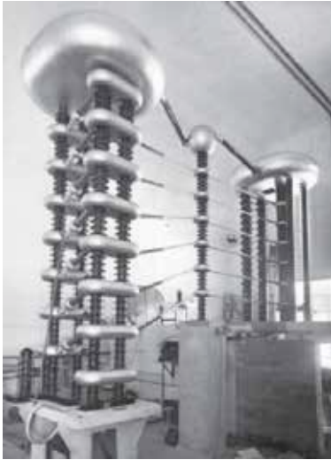
Figure 2: The Cockcroft-Walton accelerator that was moved from the Australian National University to the Physics Department at the University of New South Wales where it was used by Jak Kelly. It is an example of an early high-voltage accelerator. (ANU photo)
