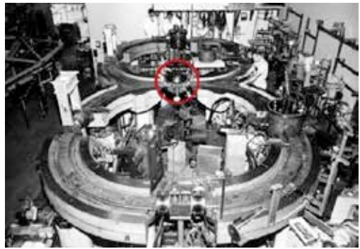
Figure 10: The Princeton-Stanford Colliding Beam Experiment used a figure eight configuration to collide 500MeV electrons.
