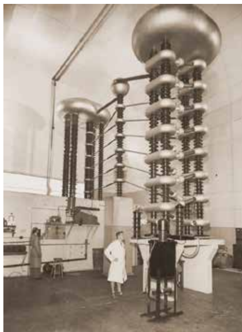
Figure 1: The 1.2 MV Cockcroft-Walton accelerator as installed at the ANU in the early 1950s. The high voltage generator stack is at the right. A uniform voltage gradient is applied to the acceleration tube via the central condenser stack. The ion source is located in the left side 'bun' at the top of the acceleration column.
