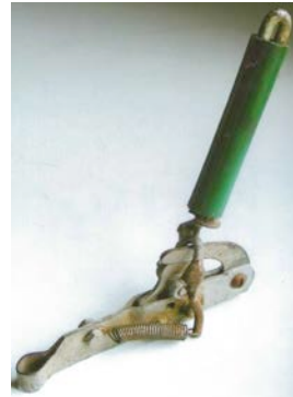
Figure 11. Release mechanism fitted to the ski boat rope attachment point to disconnect the Ski Wing in an emergency. Used from October 1963 to December 1965.
