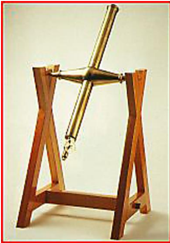
Figure 3. The 5 foot 6 inch Transit Instrument by Troughton was used to determine the position of stars for the Catalogue of 7385 Stars. The stone piers which held this instrument are to be found in Parramatta Park. The instrument is on display at Sydney Observatory.
