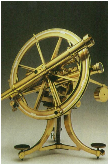
Figure 4. The 16 inch Repeating Circle by Reichenbach was located under the north dome of the Parramatta Observatory. It was used for measuring the angle between the stars for the purpose of determining their positions. This instrument is on display at Sydney Observatory.
