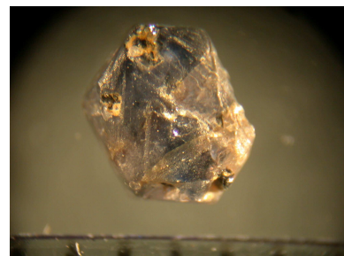
Plate 3. Pale to medium blue sapphire with several spinel inclusions. (scale is in mm).
