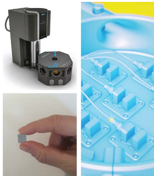
Figure 10: An NV diamond chip-set that is optically coupled, placed inside a 4K helium cryostat system.
