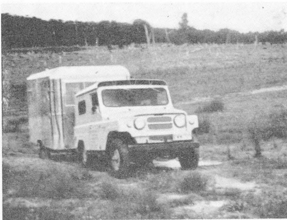
Fig. 3.—Modern mineral exploration—four-wheel-drive vehicle towing a caravan elaborately fitted out as a geochemical laboratory (after Lissiman, Baker and Marshall).
