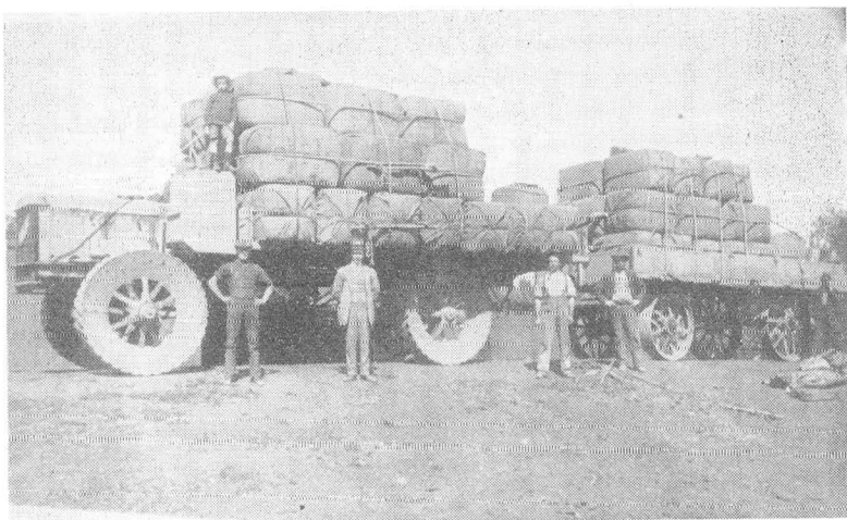
A Caldwell Vale truck manufactured in Sydney in 1909. This was the first road train in Australia and was operated by the Australian Pastoral Co. in the western part of Queensland where this photograph was taken. The vehicle had power steering, four-wheel drive and had a top speed of six miles per hour. On a test run, one of them carried eleven tons of wool up Margaret Street, Sydney, on the hill between Kent and Clarence Streets. About twenty-five of these were made and one was used by the Federal Government for the construction of the Duntroon Military College.
