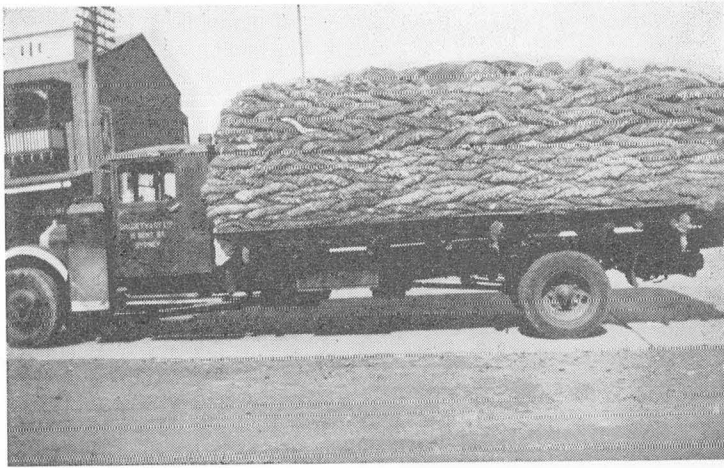
This photograph shows a gas producer unit fitted to a truck operated during the Second World War.
