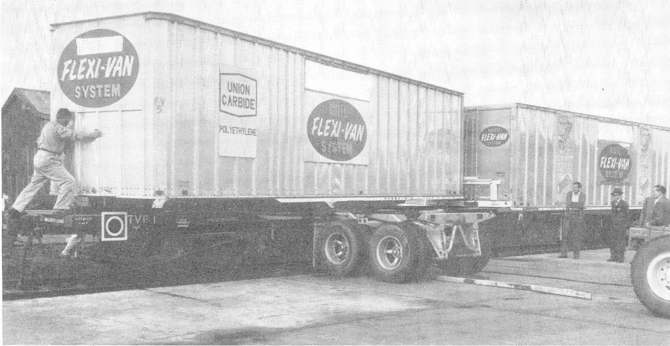
The Flexi Van. The van is mounted on a turntable on a rail truck and can be manually swung so that it can be locked on to the road vehicle before being moved away.
