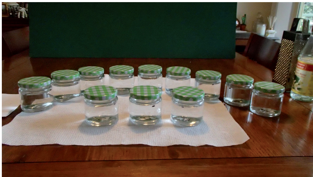
Figure 2: Jars 1 to 12 filled with a dilution series of odorant solution — in this example, rose water.
