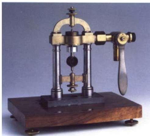
Figure 10. Foucault’s 1862 rotating mirror (the black disk at center), driven by compressed air from a pipe-organ pump. (From Tobin 1993.)
