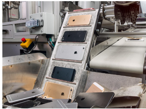
Diagram 11: Apple’s Daisy robotic iPhone cracker (Apple press release, 2018b)
