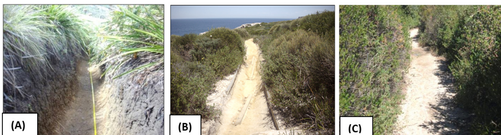
Figure 2: Examples of (A) high, (B) medium and (C) low erosion severity categories.
