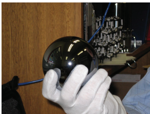
Figure 5: Walter Giardini of the National Measurement Institute Australia holding a silicon sphere as part of the Avogadro project. (photo D B Hibbert)
