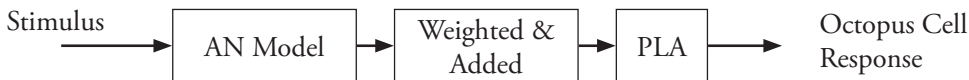
Figure 1: A schematic diagram of the model of the octopus neuron in the PVCN. The input to the model is an acoustic stimulus which is passed through the model of the AN fibre. The model AN responses for a range of CFs are weighted and added together before a power-law adaptation function is applied. The final output of the model is the simulated responses of the octopus neuron.
