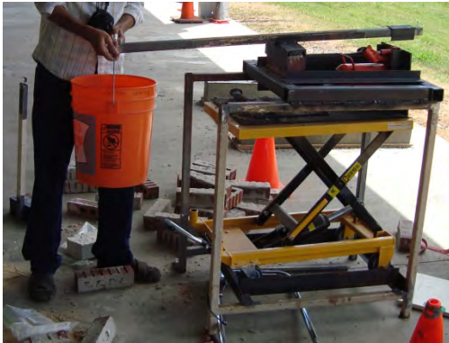
Figure 10: Balanced bond wrench and prism in testing frame.
