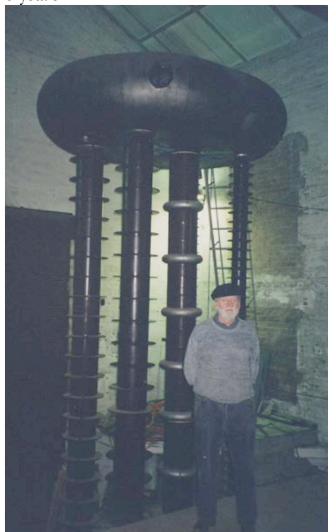
Figure 1. A thoughtful looking Jak in front of the high voltage stacks of the 1.2 megavolt accelerator at Randwick campus. Photo courtesy of Patrick McMillan.
