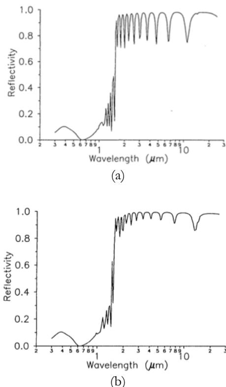
Figure 2: Modelled (a) and experimental (b) reflectivity spectra of SIM Ge/GeO<sub>2</sub> surfaces on a Cu substrate. Note the very steep edge behaviour. These figures were from Zhang, Kelly and Mills (1991). The conference paper published in 1991 included Jak's name as a co-author in recognition of his extensive work with Zhang on earlier ion beam samples which was reported.
