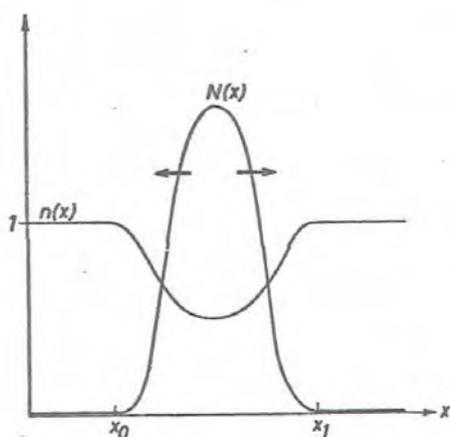
Fig. 6. Plasma layer between depths  $x_0$  and  $x_1$  with electron density  $N(x)$  and optical refractive index  $n(x)$ . The negative gradient of  $n$  causes nonlinear (ponderomotive) forces (arrows) in the space charge neutral plasma (Hora et al. 1967).
