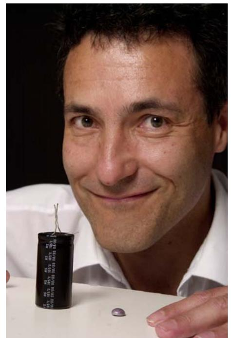
*Mike Cortie shows two capacitors. The big one is made by conventional technology and the small one has the same capacitance but is made using mesoporous gold (a sponge made of gold nanoparticles)*
